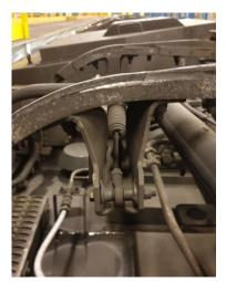
Figure 3: Broken spring box
