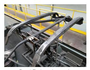
Figure 1: The damaged pantograph
