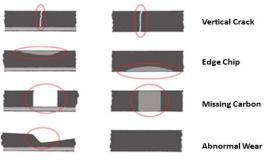
Figure 7: Carbon defect types
